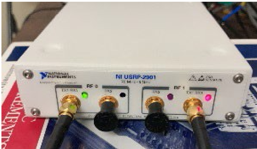
Fig. 1. The NI USRP-2901 SDR hardware in the proposed NCVS system.
