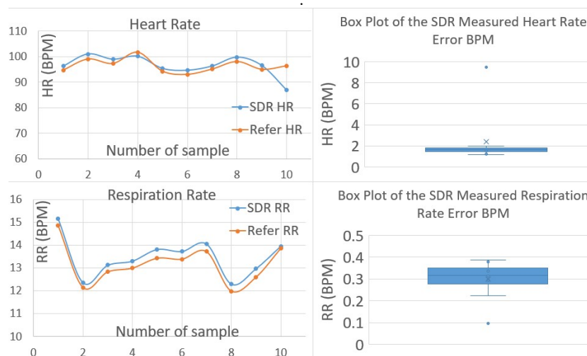
Fig. 14. Analysis of vital signs measured by our NCVS system at RX=21 (TX=21, IF=1 kHz) vs. reference signals across 10 cases (left), and boxplots of the statistics of errors from these 10 cases (right).
